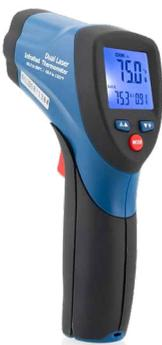
The IRT2 is a handheld, dual laser, non-contact Infrared Thermometer with 12:1 distance to spot ratio and audible and visible high/low set point alarms. It is used to measure and display surface temperatures within the range of -50°C to 650°C (-58°F to 1202°F) and has an accuracy of approximately 1 to 1.5% (see Specifications for details). The IRT2 has a fast response time (0.15 sec) and is powered with a 9V battery and complies with Class II UK/EU laser safety standard EN60285.
